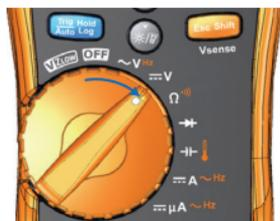
To power ON your multimeter, turn the rotary switch to any other position.
